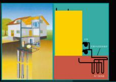
Geothermal underground loop system uses the earth's constant temperature to exchange energy between the earth and your building. Energy is collected through pipes installed in the ground called loops. There are several loop configurations vertical, horizontal, or submerged in pond or lake. The configuration of your property will
